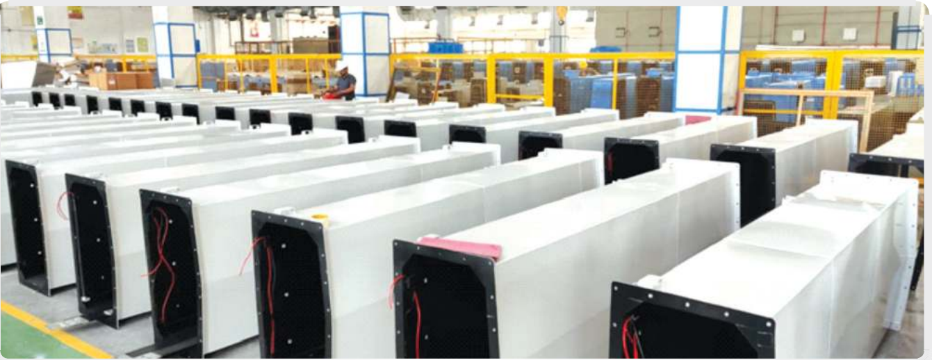
Bus Duct ready for Dispatch
