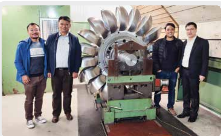
FAT of the Pelton Runner at the Manufacturer's Factory
